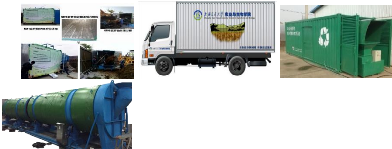
Figure 4. System equipment for straw fermentation. (a) first generation equipment, demonstrated in Chongming Zhongxin Taisheng Farm, Shanghai, (b) second generation equipment, demonstrated in Pujiang Green Valley Practice Base, Shanghai, (c) third generation equipment, demonstrated in Chongming Lvru fruit and vegetable Specialized Cooperative (Maqiao Base), Shanghai, (d) fourth generation equipment, demonstrated in Chongming Xiangnong Specialized Cooperative.
